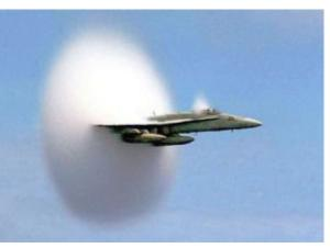
and A commonly encountered shock wave is USA the have the sonic shock produced by supersonic Australia. Spitzer aircraft, such as this US navy jet on a fast the turned Telescope, low flyby over the sea. As a supersonic jet Space a exceeds the speed of sound (or Mach 1), it with equipped catches up with its own sound waves. The super-sensitive sound waves become compressed infrared together into a cone-shaped "shock" which spectrograph, towards the location travels outwards towards the ground,
