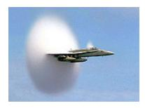
A U.S. Navy fighter jet breaks the sound barrier, creating a shock wave. Credit: Courtesy of the U.S. Navy
