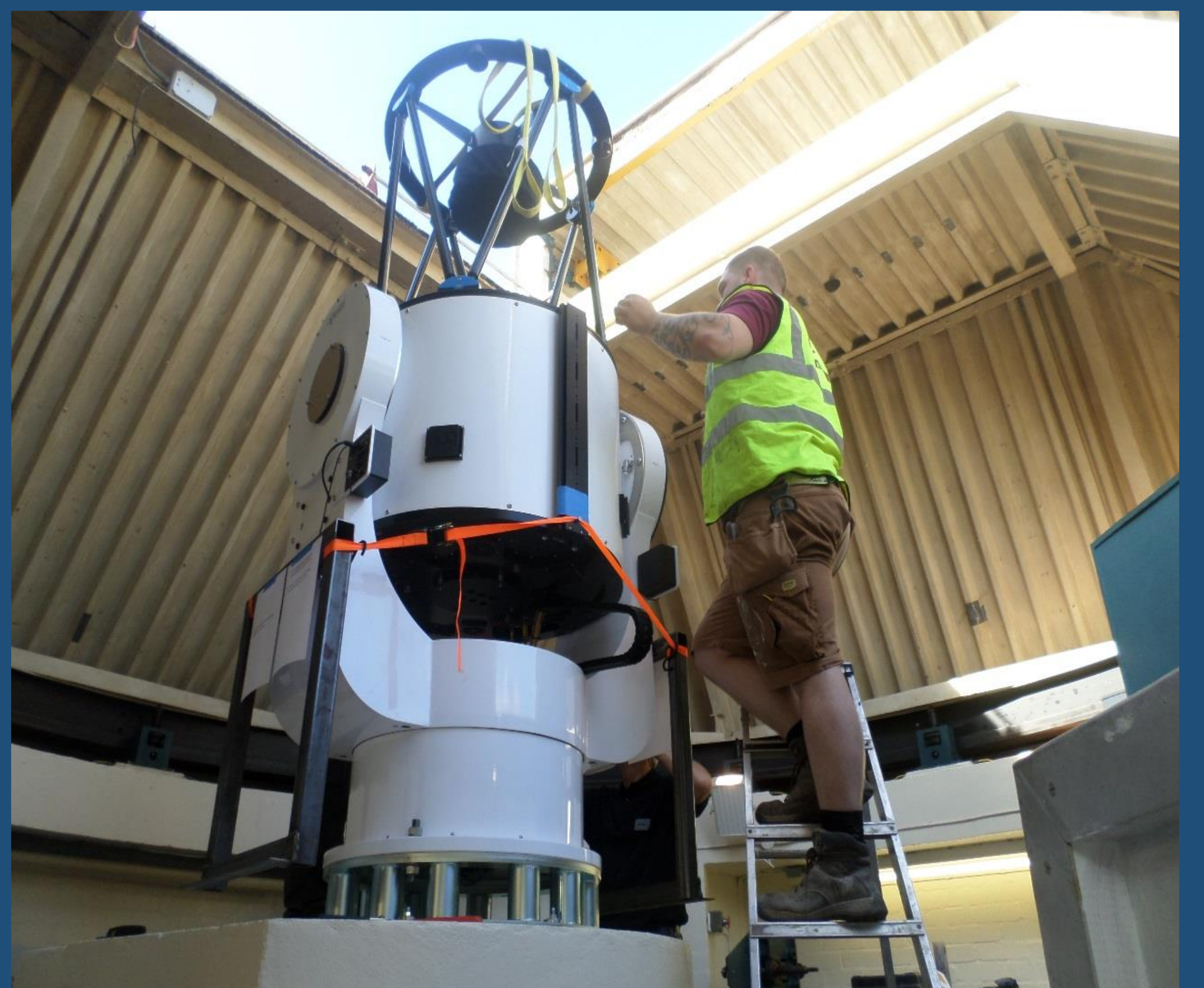
Figure 3: The upper section of the telescope, including the secondary mirror, is lowered carefully into position. The Nasmyth focus can be seen on the axis of the elevation drive. There is another focus on the opposite side, and the tertiary mirror can be rotated to access either side.
